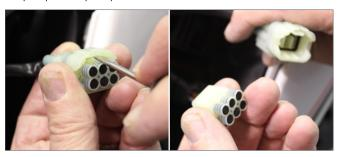
**3.** Connect the MagVolt® TPS power lead to the diagnostic port and re-install it on its mounting tab.
