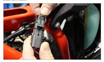
5. Connect the white 3-pin TPS connector to the wiring harness where the stock connector used to be.
