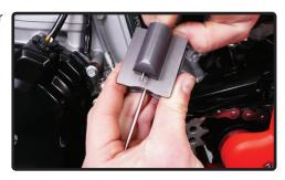
E. Once the cable end is through the large hole in the bottom of the slide's nose, push it over into the smaller retaining hole and carefully let the throttle return spring and cable retainer relax
