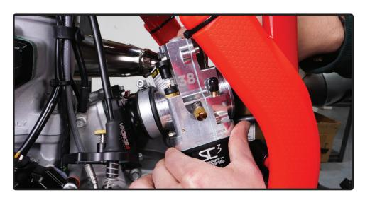
**B.** Check for pinching or distortion of the airboot. Remove the filter and look down through the airboot to ensure that the rubber is not collapsed and that the Vent Scoop located in the top of the venturi is clear and unobstructed.
