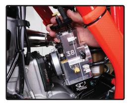
D. Rotate the mounted SmartCarb® to where it is as straight upright as possible and tighten the hose clamps on the intake manifold and the airboot. Make sure that the SmartCarb® is not touching any hard surface and that the Float Bowl cannot come into contact with the chain during operation of the vehicle.
