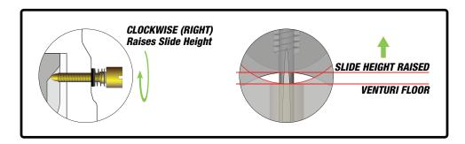
Turning the screw out counterclockwise to the left will lower the slide height:
