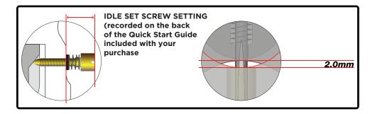
A 2.0mm slide height maximizes the signal through the venturi for high air velocity, brings the engine down smoothly back to idle when the throttle is closed, and improves cold starting by letting most of the air pass through the Choke circuit providing proper cold start enrichment and high idle warm-up.
