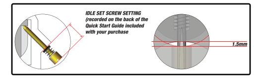
A 1.5mm slide height maximizes the signal through the venturi for high air velocity, brings the engine down smoothly back to idle when the throttle is closed, and improves cold starting by letting most of the air pass through the Choke circuit providing proper cold start enrichment and high idle warm-up.
