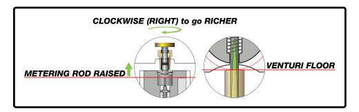
Adjusting the Clicker Adjuster to the left, or counterclockwise, will lower the metering rod within the slide. Lowering the metering rod will reduce fuel being added to the mixture as it exposes less of the angled surface grind of the metering rod.
