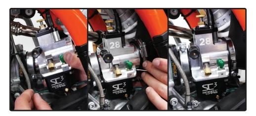
**B.** Once installed, check for pinching or distortion of the airbox or airboot. Remove the filter and look down through your airbox and make sure that the rubber is not collapsed and that the Vent Scoop located in the top of the SmartCarb® carburetor's venturi is clear and unobstructed. Reaching into the airbox with a mirror or using a camera may be required. Trimming of the airbox or airboot may be required.
