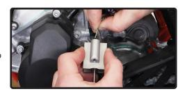
E. Hold the spring and cable retainer back and insert the cable end through the large hole in the bottom of the slide's nose.
