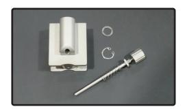
**G.** Unscrew the adjuster or clicker barrel from the metering rod.
