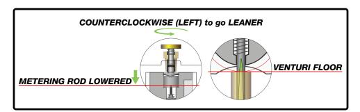
A simple rule of thumb is to turn Right for Richer and Left for Leaner.
