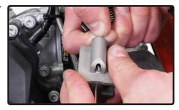
E. Once the cable end is through the large hole in the bottom of the slide's nose, push it over into the smaller retaining hole and carefully let the throttle return spring and cable retainer relax
