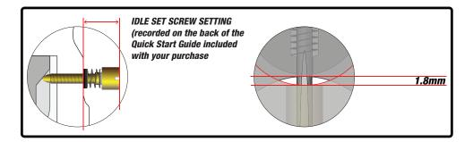
A 1.8mm slide height maximizes the signal through the venturi for high air velocity, brings the engine down smoothly back to idle when the throttle is closed, and improves cold starting by letting most of the air pass through the Choke circuit providing proper cold start enrichment and high idle warm-up.
