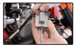
F. Once the cable end is through the large hole in the bottom of the slide's nose, push it over into the smaller retaining hole and carefully let the throttle return spring and cable retainer relax
