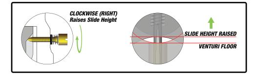
Turning the screw out counterclockwise to the left will lower the slide height:
