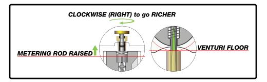
Adjusting the Clicker Adjuster to the left, or counterclockwise, will lower the metering rod within the slide. Lowering the metering rod will reduce fuel being added to the mixture as it exposes less of the angled surface grind of the metering rod.
