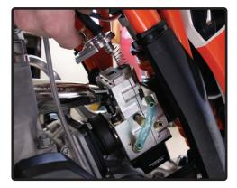
D. Rotate the mounted SmartCarb<sup>®</sup> to where it is as straight upright as possible and tighten the hose clamps on the intake manifold and the airboot. Make sure that the SmartCarb<sup>®</sup> is not touching any hard surface and that the Float Bowl cannot come into contact with the chain during operation of the vehicle.
