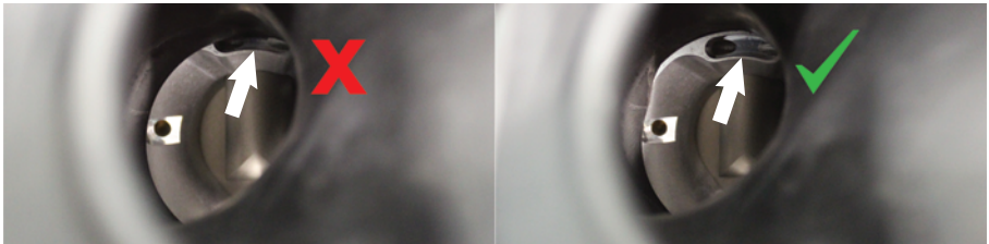
SmartCarb® venturi as viewed through the airboot.
